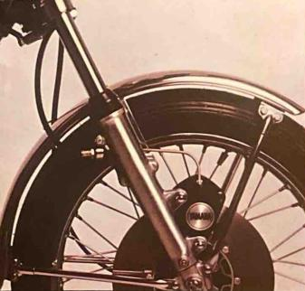
Front disc brake stops you faster. An adjustment screw lets you set the hand-lever for the exact "feel" you prefer. The enduro-type front forks will soak up the hardest jolts. Without bottoming.
