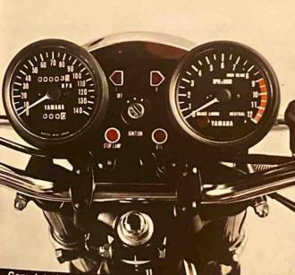
Complete instrumentation includes fully illuminated speedometer and tachmeter. Warning lights provide a constant check on turn signals, tail lights..even rear brake lining wear and oil pressure, on some models.
