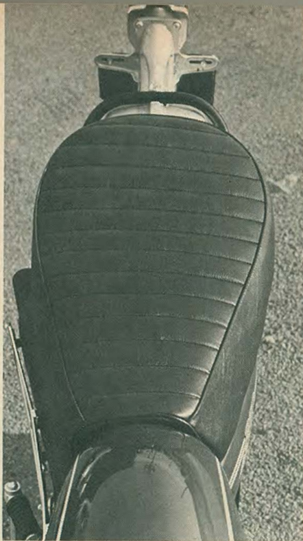
The saddle provided maximum comfort. The high tail light is one area that could use redesigning as it catches the leg when mounting the machine.
