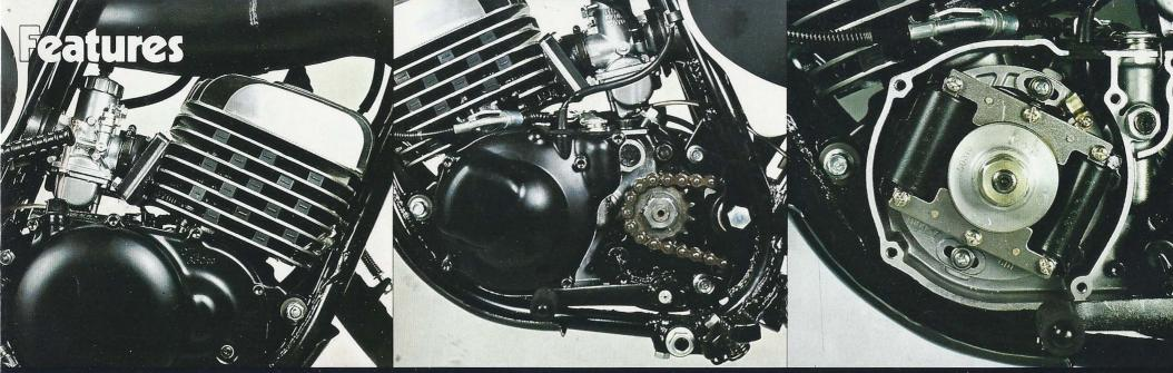
**Torque Induction,** Yamaha's unique reed-valve intake system, feeds the engine the exact mixture of fuel and air it needs. The result is more horsepower, particularly at low rpm's.
