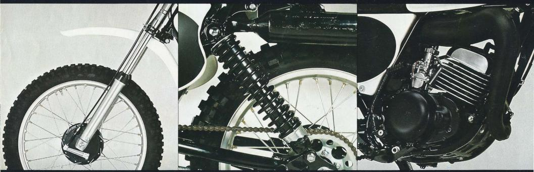
**Longer travel, heavy-duty front forks** soak up sharp jolts without bottoming. Lightweight polypropylene fenders are virtually unbreakable and conical hubs help reduce unsprung weight. Forward-mounted nitrogen/fluid shocks provide greater rear wheel travel for better control, consistent traction and superior fade-resistant damping.
