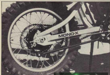
This will probably be the last year you'll see the trademark Yamaha Monoshock design. The factories are playing with a progressive setup similar to the Honda Pro-Links.
