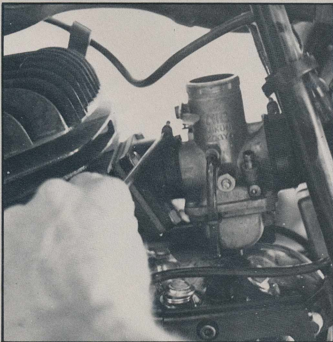
Stock hoses and clamps can be used. Make sure you don't overtighten the clamps, which will rip the hose and cause an air leak in the system.
