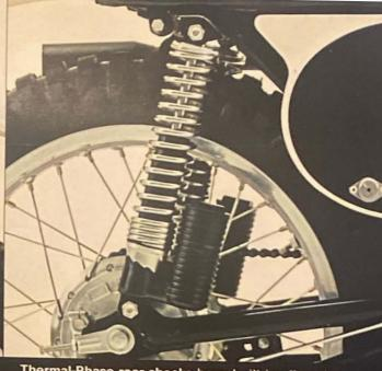
Thermal-Phase rear shocks have built-in oil coolers to prevent overheating no matter how hard or long you ride.
