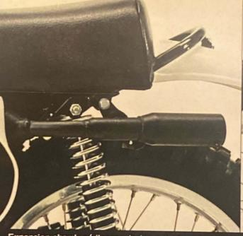
Expansion chamber/silencer design cuts down noise without cutting down power. Over-the-top configuration results in better road clearance, less chance of burns.
