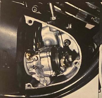
Autolube constantly adjusts the flow of oil into the fuel mixture according to engine load and speed, resulting in increased engine life. For those who want to save a little weight and premix, the unit is easily detachable.
