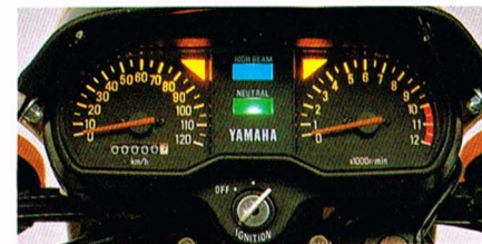
As you would expect on a sports motorcycle, the RD80MX is fitted with a large rev-counter to match the easy to read illuminated speedometer. The instrument console also includes a neutral indicator and high beam lamp.
