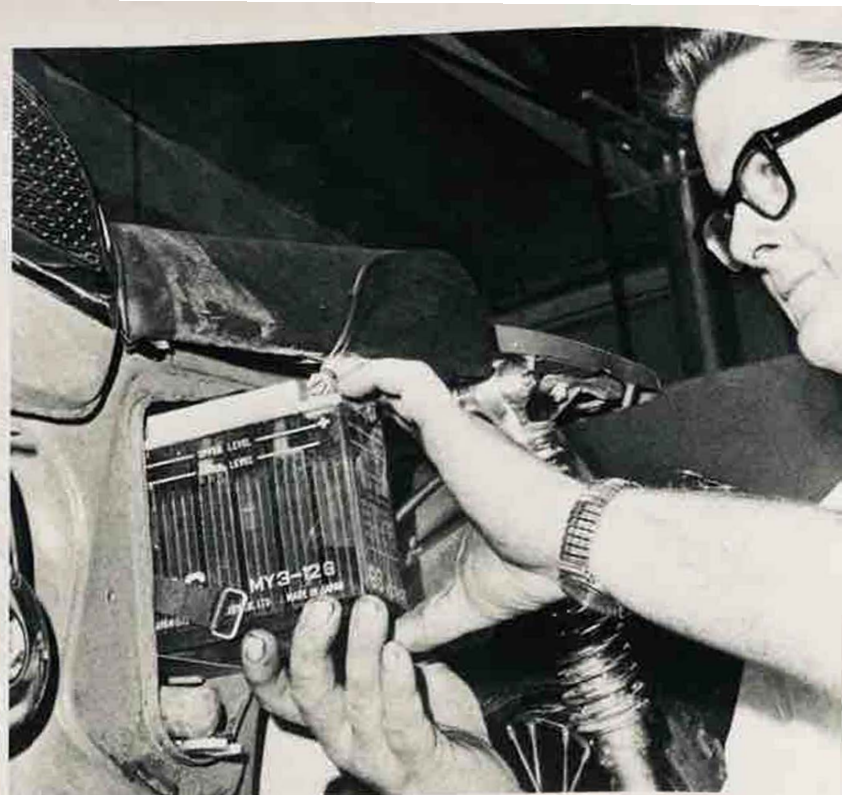
Twelve-volt System is new Yamaha feature. Big battery has ample reserve and lights are bright when engine is not running.
