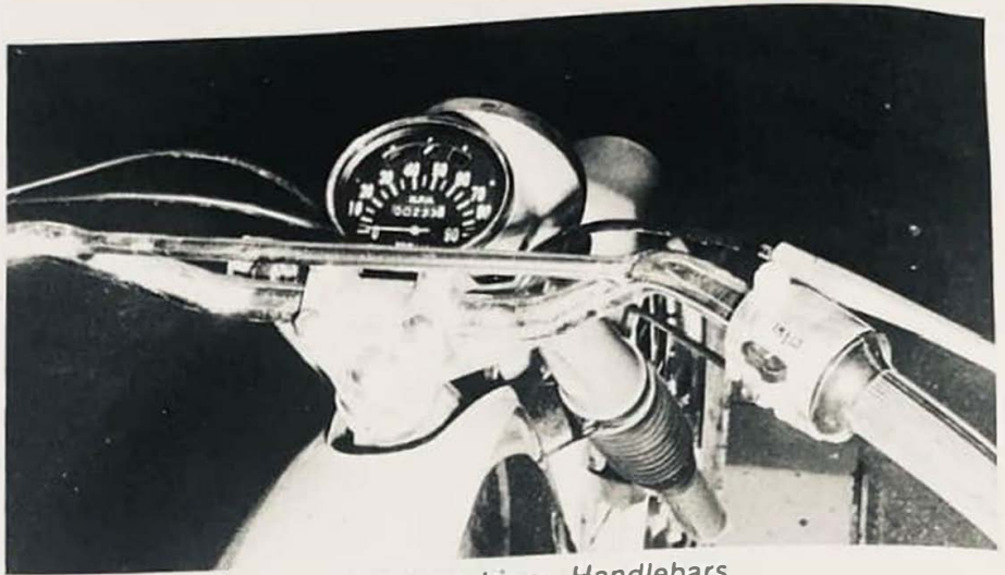
Speedometer has big, readable markings. Handlebars have designed-in crossbar. Emphasis seems to be on function throughout.
