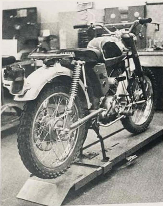
Prototype model spent much time in Yamaha shop being modified. Factory has incorporated changes into production versions.
