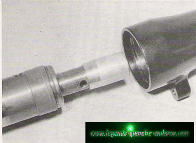
5.7c ... and slide into lower leg
