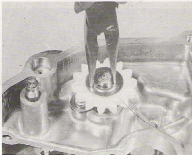
25.2f Retain the assembly with the plain washer and circlip
