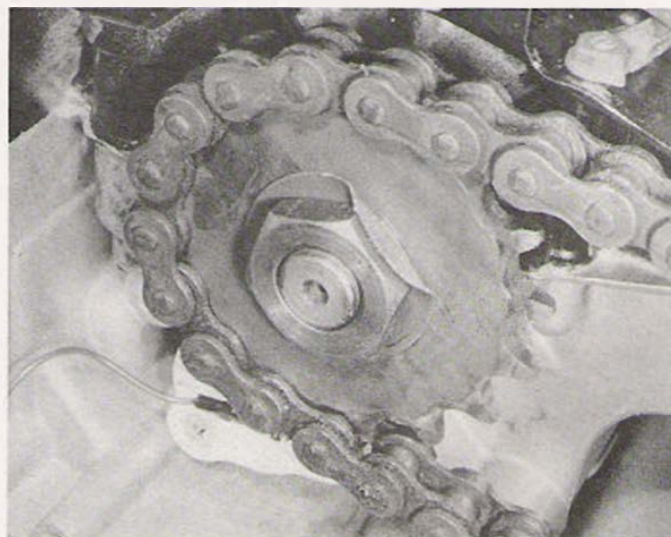
35.4c ... tighten securely and bend up the locking tab as shown
