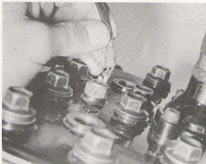
4.5b Disconnect the water temperature sender lead
