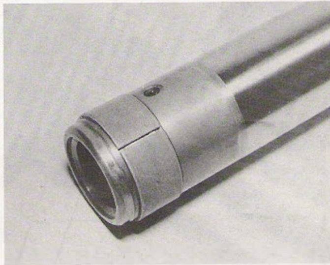
5.6 Bottom bush is split to facilitate removal – do not stretch new bush more than absolutely necessary during fitting
