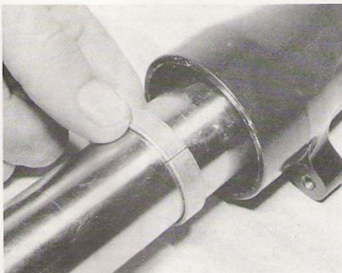
5.8a Lubricate top bush and slide into place
