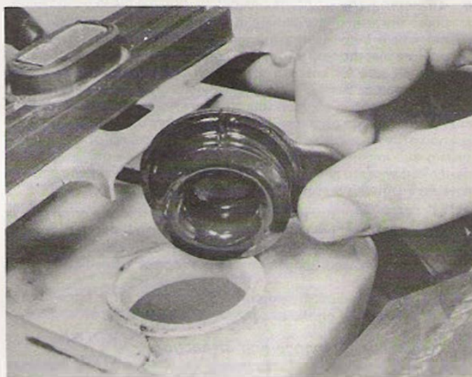
Engine oil tank filler can be reached after seat has been removed
