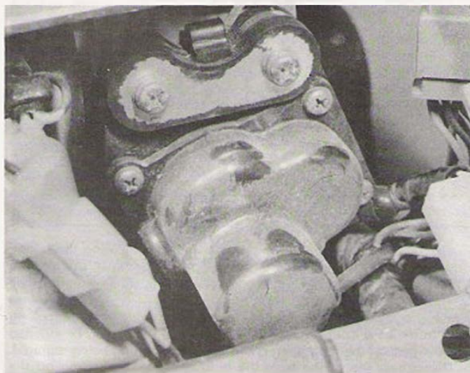
8.2a The YPVS servomotor is located to the rear of the steering head
