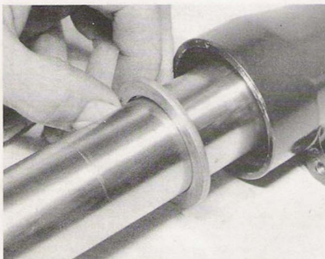
5.8b Fit plain washer and tap bush into top of lower leg
