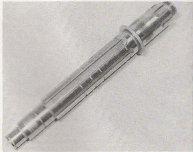
14.7a The output shaft has a plain shoulder at the left-hand end
