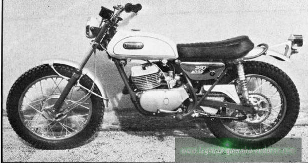
Hit of the Yamaha exhibit was the new DT1 Trail machine, reported to develop 19 bhp at 6000 rpm with its 246-cc engine. Claimed weight is 220 lb.
