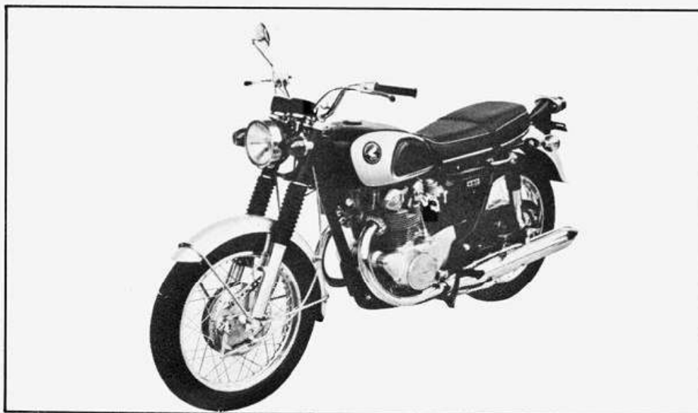
The new, lithe Honda CB450 is much slicker looking than its predecessors, boasts 45 bhp at 9000 rpm, 112-mph top speed, and a swift quarter-mile.
