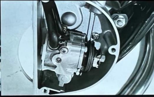
Autolube. a feature on most Yamaha two-stroke engines, automatically injects oil into the fuel mixture, eliminating the need for premixing. And, since it adjusts the flow of oil to engine load and speed, it extends engine life.
