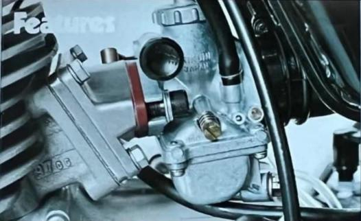
Torque Induction, Yamaha's unique intake system, utilizes a reed valve to feed the engine the exact amount of fuel and air it needs. The result is that horsepower is increased, particularly at low rpm's.
