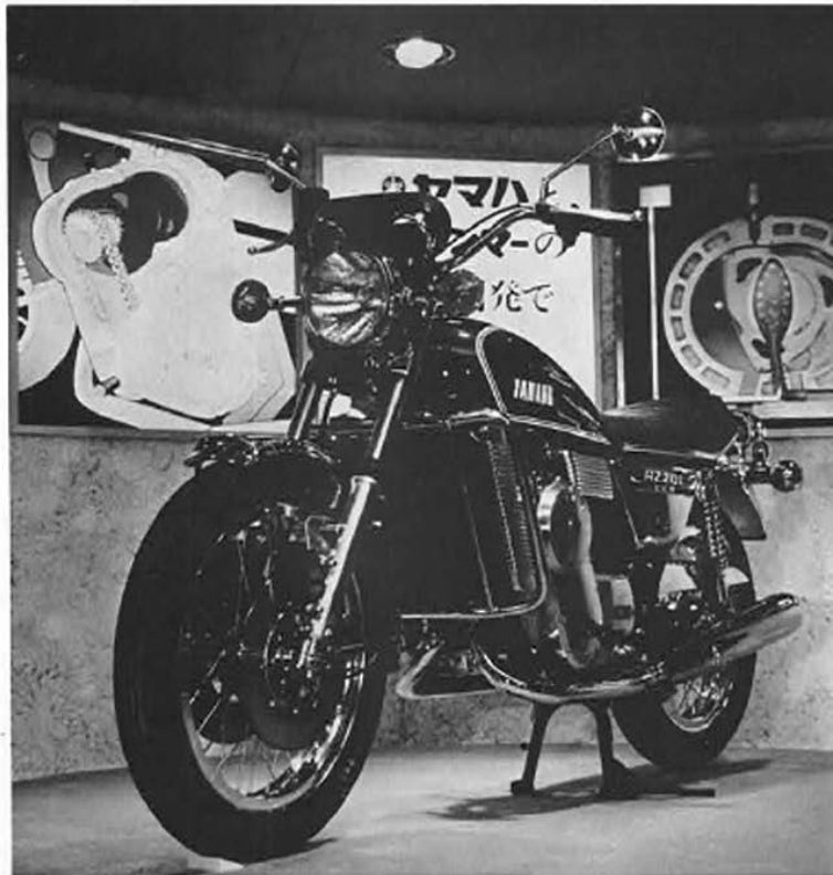
Photo: The Yamaha Rotary RZ200, the first rotary engine motorcycle prototype ever built in the world with the definite intention of mass production, made a quiet but sensational debut at the '72 Tokyo Motor Show. Yamaha has successfully consolidated all proven technical merits into this model, as represented by the in-line twin rotor revolving in the same direction as that of vehicle advance, VCR system, peripheral parts, etc. The age of rotaryization is about to open with Yamaha.
