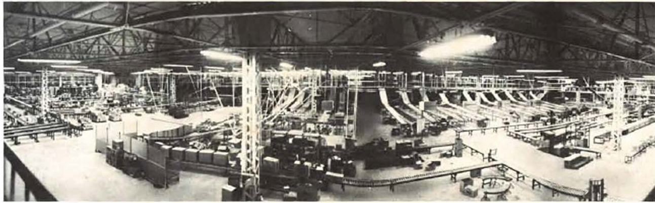
Conveyor system. Every shifting process from incoming down to outgoing parts performed on efficient conveyor systems.
