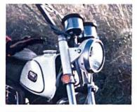
RUGGED TRAIL FEATURES These include a sturdy lightweight frame, special travel forks, engine guard, a maximum amount of ground clearance, large non-slip seat and separate tachometer and speedometer instruments.
