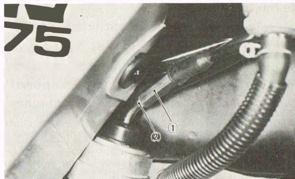
1. Adjuster 2. Lock nut
