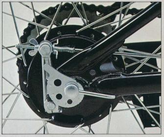
**Chain-adjusting cams** allow rapid rear wheel alignment when adjusting the drive chain or after removing the rear wheel.
