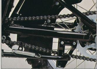
**Chain shield** keeps mud and sand from being thrown into the chain. Increases chain life.
