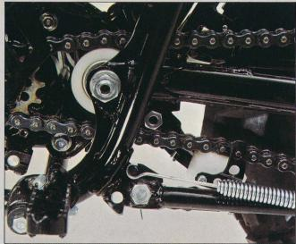
**Spring-loaded chain tensioner** helps to maintain an even chain tension and perfect adjustment even under extreme conditions.
