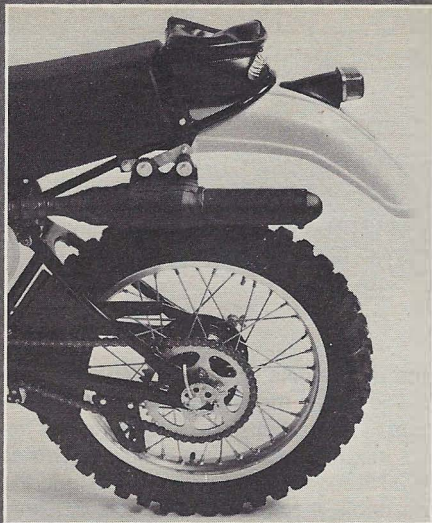
Tools need more secure mounting inside pouch. USFS spark arrestor and silencer are effective.
