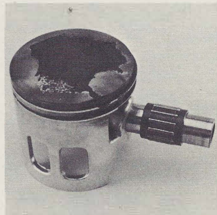
Piston crown showed only moderate carbon build-up. Two keystone rings and needle bearing are standard.
